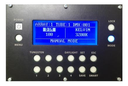
Each **ARRAY** consists of a set of four tubes. You have the ability to control each individual tube within each **ARRAY** (see page 4). Depending on your fixture model you could have anywhere from 1-5 **ARRAYS**.
